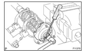
(c) Using a screwdriver to hold the spring seat, remove the nut.
